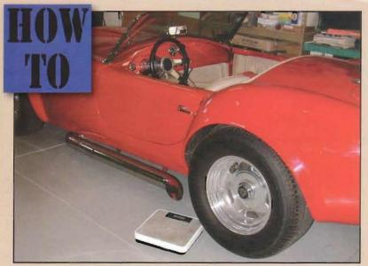
You can't just ask your car to hop up on the bathroom scale, but there is an easy way to calculate the weight of your car by using little more than a tire gauge, tape measure and a couple of straight edges.
