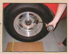
the amount of weight that the tire is supporting. Repeat the steps above for every tire and add all the results to determine the weight of your car. Air pressure is measured by how much weight it can hold up. In fact, if you look on the sidewall of your tires, there will be a maximum weight rating for the tire.
