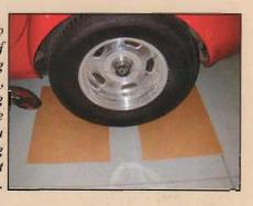
With the cardboard pieces parallel, measure the foreand-aft dimension then the side-to-side dimension. When you multiply those two measurements you have the surface area of the contact patch in square inches.
