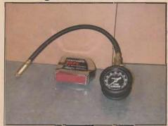
The tools for this simple weighing project are minimal, requiring only two pieces of cardboard with straight edges, a tape measure and a tire pressure gauge that measures in pounds per square inch (psi).
