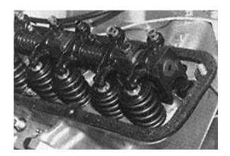
Ford Power Parts rocker shafts and stands were used in the stock 1.76:1 ratio. The solid lifter cam's valve lash (hot) is .018-inch intake and .020 exhaust. New, genuine Ford push rods, with oval and cupstyle ends, were fitted. The Iskenderian valve springs have an installed height of 1.875 inches. ARP head bolts were used and torqued to 100 lb ft of torque.
