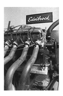
Edelbrock's dyno header's primary tubes were large 2.125-inch-diameter monsters; all in the name of accommodating the 6500 rpm exhaust flow. The engine was tested without mufflers. **SF**
