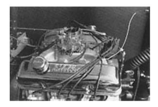
Edelbrock's Performer Series 750 cfm carb was tested and only metering rods and jets were changed to provide optimum air/ fuel calibration for this engine. This carb has a one-piece top, which facilities easy jet changes and eliminates gaskets below the fuel line to help prevent leaks. The distributor is a stock Duraspark unit.
