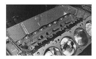
The block valley has been coated with Gyptal paint, which seals the casting surface to aid oil drain-back. JE pistons are a flat-top configuration with two intake valve reliefs and they run with .0025 of an inch piston-to-wall clearance. Deck clearance was .007 of an inch in the hole.
