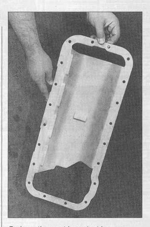
Perhaps the most important improvement you can make to your 390/428 FE engine is the installation of a 427/428SCJ-style windage tray. Dollar for dollar this is the cheapest horsepower you can buy. On engines revving over 6000 rpm, gains from 10 to 15 horsepower can be expected. The windage tray prevents the spinning crank from sucking up oil from the sump, which slows down the crank.
