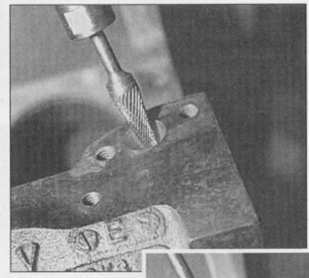
After using the FPP gasket to scribe the orifice, use the carbide bit to increase the size and use the cartridge roll to polish and remove all excess burrs.
