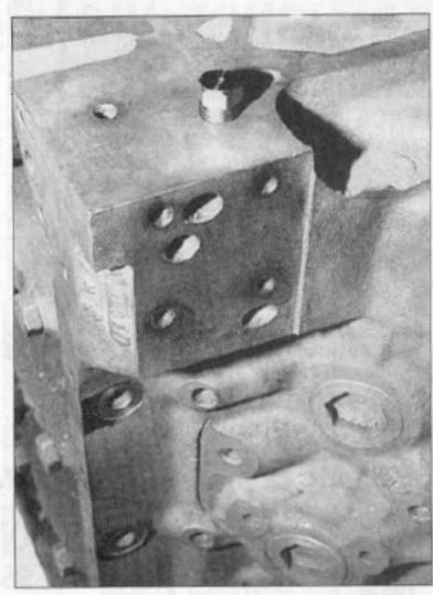
Never available separately from Ford, FPP is now offering an exact reproduction of this uniquely threaded special plug that goes at the front of the side oiler passage. In the past, if you didn't have this plug, a used original one would cost from \$20 to \$40—and that's if you could find one! FPP sells a reproduction of this plug for only \$11.95.
