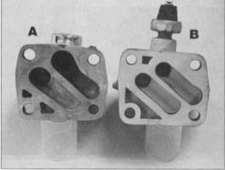
Polish the two openings using a cartridge roll until smooth. After this area is done, inspect the block for any sharp edges and/or burrs. Deburring the block is important to
