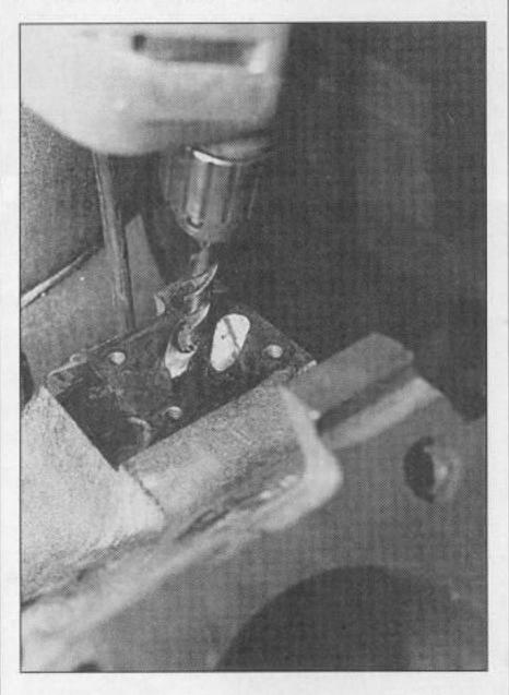
All FE blocks (except 406 and 427) have a very small %-inch-diameter hole from the oil pump to the oil filter adapter. FPP drills this out (from the adapter side) to ½ in ¼-inch increments. Starting with ¼ inch, move up to ½, then ¼, and finally ¼ inch. Use a heavy-duty ½-inch chuck drill and be careful at the end of drilling to prevent the drill bit from chipping or breaking a piece of the block where the oil pump mounts.
