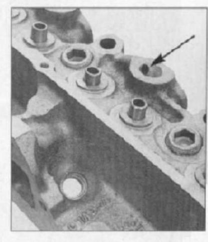
inch. The big valve FE heads (427 Medium Riser, High Riser, and Tunnel Port) have a smaller passage of .250 inch. The result is less oil to the top end and more oil to the crank. Does .090 inch seem too small to feed an entire rocker assembly? With the oil hot, remove one valve cover and rev the engine to 4000rpm and watch the amount of oil on the top end. For dragrace-only FEs, builders often restrict this orifice to only .060 inch.
