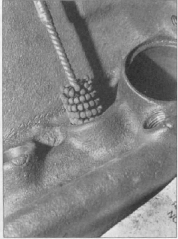
Once the front gallery plug orifice is threaded, it is a good practice to ball hone the lifter bore to ensure that no burrs are protruding into the lifter bore. Check the other 15 lifter bores to ensure that a lightly oiled lifter slides easily in and out of each bore.
