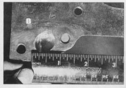
Look at the difference between the before and after pictures. The idea is for the oil to flow throughout the entire block without any obstructions or sharp turns. Not only is volume increased by doing this, but the oil is cooler as well.
