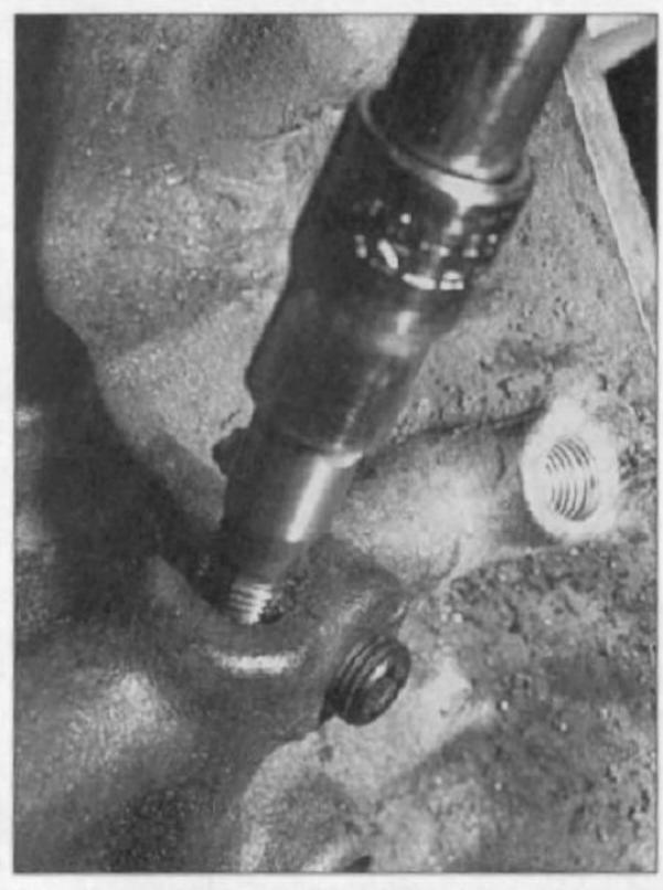
The internal gallery press-in plugs are replaced with screw-in 1/4-inch NPT plugs. Never install oil gallery plugs dry. Using liquid Teflon® works as both thread lubricant
