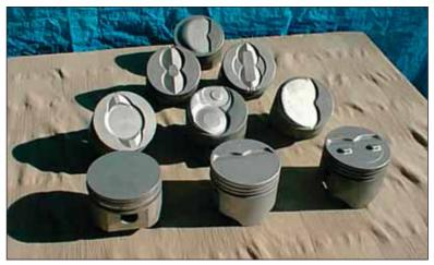
These are just nine of the variations of FE pistons. Depending on the head, the compression ratio, and the valve size, you could end up with any of them. Most are obsolete and in some cases result in too much compression to run today's fuels. All are obsolete designs that are not well suited for modern performance.
