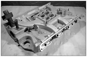
FE intakes form the inner side of the heads so sealing between the head and intake is critical. These are very large items and the cast iron versions required the use of a cherry picker to remove from the engine compartment. There were some aluminum performance intakes from Ford.
