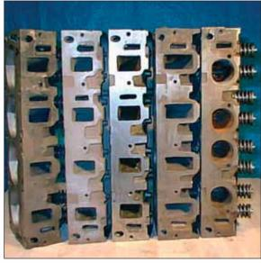
Stock FE heads came in several different variations. They go from mild passenger heads to performance and right out to race style (for the day) heads that are quite rare now. For restorations and mild-to-moderate performance, you can still use stock cast iron heads. Valve re-sizing and porting do a lot of good for any of them.
