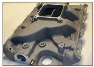
Aftermarket aluminum intakes do two important things for the FE. First, is the obvious performance improvements in flow and velocity. Second is the significant decrease in engine weight. An FE can easily be in the small block Chevy weight range with aluminum heads and intake.
