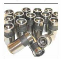
Original flat-tappet lifters have occasionally been hard to find lately as the manufacturers changed to later engines and rollers. Fortunately you can still get OEM replacements in good supply
