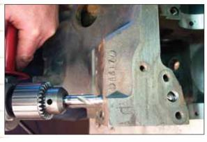
In original blocks, one of the key modifications used to improve oiling for performance engines is to enlarge the oil pump to filter passage. Look for tech sources like WebRodder.com to make sure you have the details of these operations so you can offer them to your customers and build better engines.
