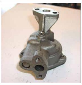
There are several versions of FE oil pumps that range from street stock on up to high pressure side oiler units. FE engines need all the oil they can get so the high volume pumps are best, but the high pressure pumps are ONLY for the side oiler engines. High pressure does NOT translate to good flow.
