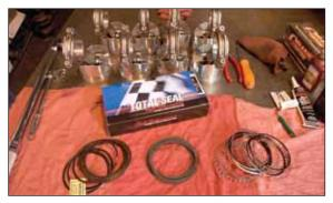
My research tells me that FE engines LOVE stroke. A stroker kit can make a number of improvements all at once including better, lighter pistons with modern thin rings, better rods and rod ratios, and more cubes. Remember for ultimate performance it's either cubic inches or cubic dollars!
