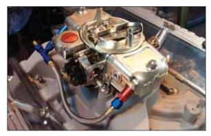
If you are not doing a restoration, carburetion is an issue. We did a bunch of experimenting on the dyno with carbs and the Barry Grant Demon carb was the best of those tested. We were surprised to find that this 750 cfm unit made better power than an identical 850 cfm unit on the dyno. This from an engine putting out over 450 hp and 500 ft.lbs. of torque.
