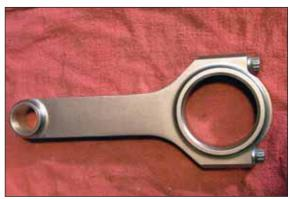
The Eagle H-beam rods are also a great asset in an FE engine. Often part of a stroker kit, they allow you to alter the rod length and get better internal geometry. FE engines like long arms.
