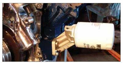
Part of making an FE suitable for a specific customer application is knowing which parts work best. If you have lots of side room, but little between frame and block, you might opt for this style oil filter housing, for example.
