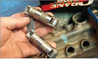
I found that the best performance – showing flat and high torque and horsepower curves – of any cam combination for the street came from Crane Cams' street grind roller hydraulic cams. This was another of those dramatic improvements we found for the FE. The roller cams really help them breathe better and the hydraulics make them streetable without a lot of maintenance.
