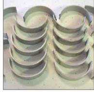
Rod bearings are available in all standard oversizes and in various material and construction styles. Egge offers them for all FE engines back to the first 1958 332.
