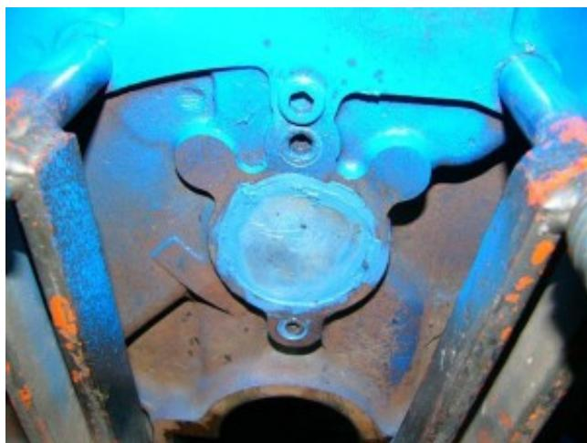
Another important note — The rear cam plug on FE Fords is faced with cup inward to give it cam butt clearance.
