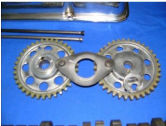
Good view of the early flat rear, upper timing gear on the right, with the needed remote .222 thick steel spacer. The later upper timing on left has the spacer molded on the back. Do not mix these up. Never use the remote spacer with the late spacer step molded gear. The steel retainer was used on both types from 1963 on.
