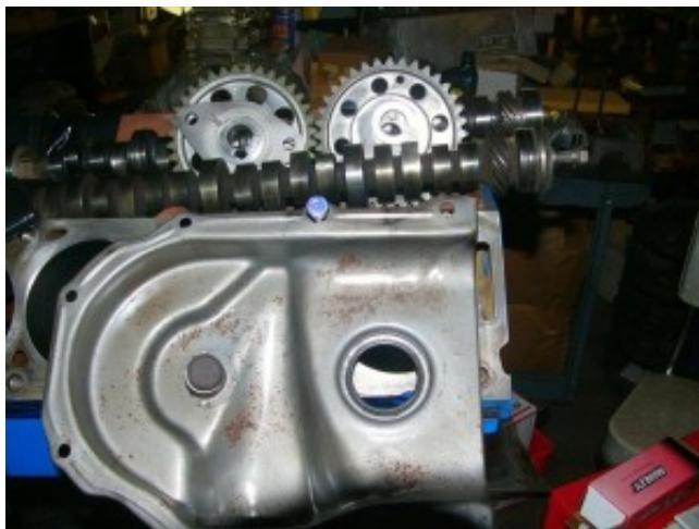
1958-1962 FE engines had cams, like the one pictured, just above the front cover. That big flange rode on front of the block. The cam was retained with spring in special steel front cover as pictured here. In 1963, Ford switched to a non-flanged cam and retaining plate with a more modern timing gear.
